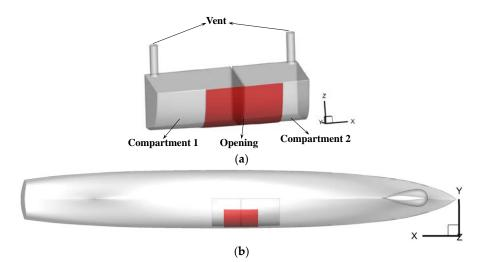
**Figure 2.** Model of frigate with damaged compartments for asymmetric flooding: (**a**) Compartments (**b**) Ship.
