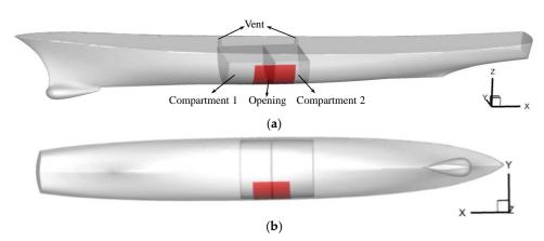
**Figure 1.** Model of frigate with damaged compartments for symmetrical flooding at different views: (a) Side view (b) Bottom view.
