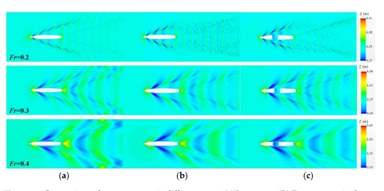
**Figure 15.** Comparison of wave patterns in different cases: (**a**) Intact case; (**b**) Damage-repaired case; (**c**) Symmetrical flooding case.
