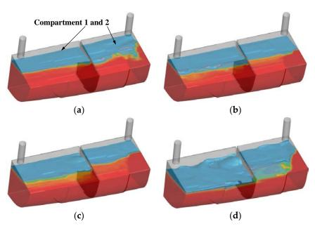
**Figure 19.** Comparison of water surface in compartments for the ship under asymmetric flooding at different speeds: (a) Fr = 0.1 (b) Fr = 0.2 (c) Fr = 0.3 (d) Fr = 0.4.
