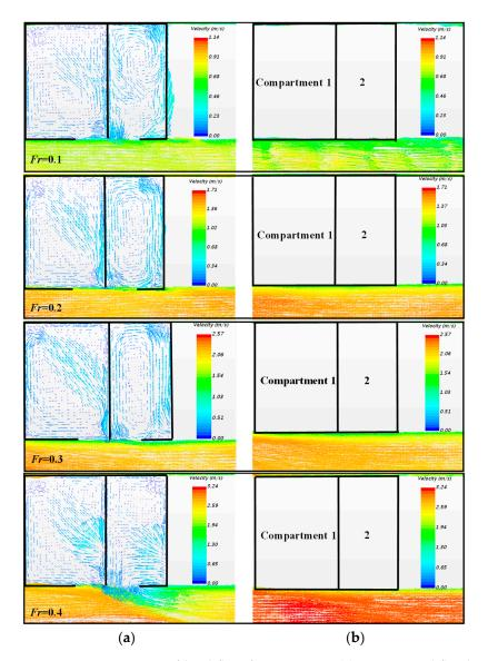
Figure 16. Comparison of local flow for two cases: (a) Symmetrical flooding case; (b) Damage-repaired case.
