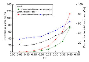
**Figure 13.** Comparison of pressure resistance and its proportion to total resistance for the ship in intact and symmetrical flooding cases.
