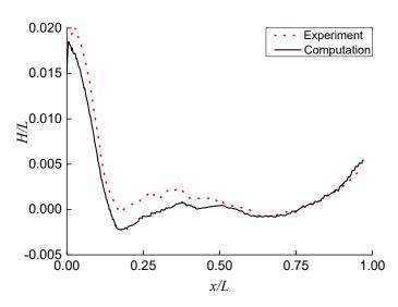
**Figure 6.** Comparison of wave elevation on hull surface obtained by computation and experiment for intact ship.
