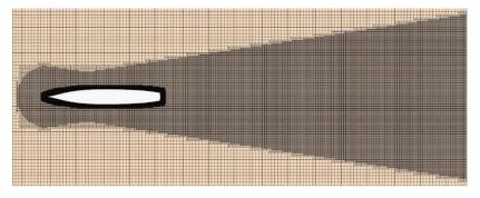
Figure 4. Mesh arrangement for intact ship case (medium mesh).
