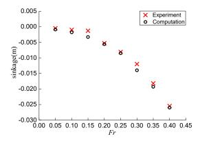
**Figure 10.** Comparison of sinkage obtained by computation and experiment for intact ship at different forward speeds.
