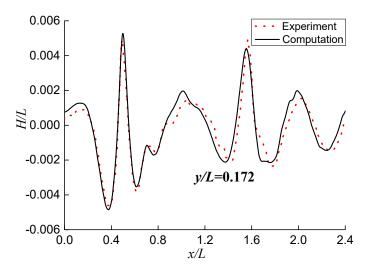
**Figure 8.** Comparison of wave elevation at y/L = 0.172 longitudinal section obtained by computation and experiment for intact ship.
