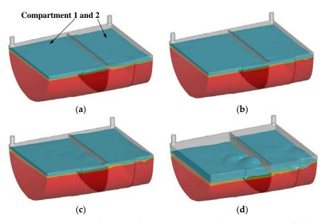
**Figure 17.** Comparison of water surface in compartments during symmetrical flooding at different forward speeds: (a) Fr = 0.1 (b) Fr = 0.2 (c) Fr = 0.3 (d) Fr = 0.4.
