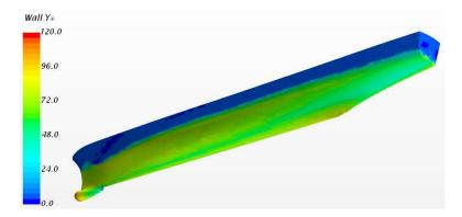
**Figure 5.** *Y*+ distribution on the hull for medium mesh.
