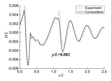
**Figure 7.** Comparison of wave elevation at y/L = 0.082 longitudinal section obtained by computation and experiment for intact ship.
