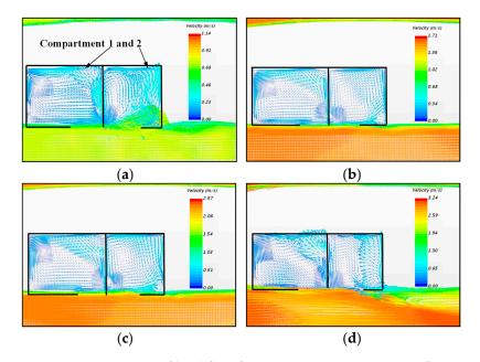
**Figure 18.** Comparison of local flow for the ship under asymmetric flooding at different forward speeds: (a) Fr = 0.1 (b) Fr = 0.2 (c) Fr = 0.3 (d) Fr = 0.4.
