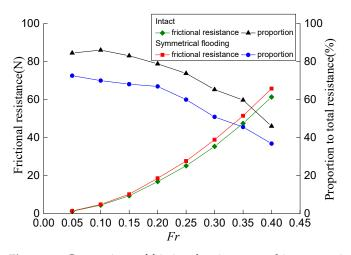
**Figure 12.** Comparison of frictional resistance and its proportion to total resistance for the ship in intact and symmetrical flooding cases.
