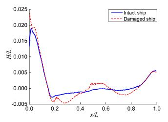
Figure 14. Comparison of wave elevation on the hull surface for intact and damaged ships (*Fr* = 0.30).
