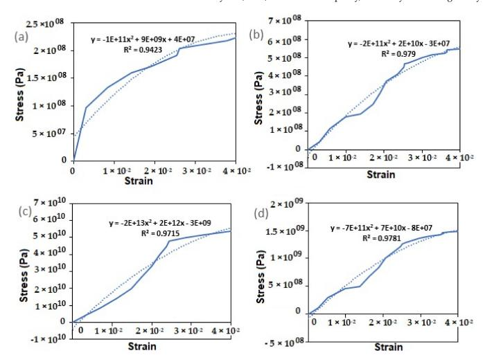
**Figure 14.** Stress–strain relationships for total strain in XX direction showing (**a**) elastoplastic material model, (**b**) epoxy linear elastic model, (**c**) carbon fibre linear elastic model and (**d**) Nylon PA66-Glass Fibre linear elastic model.
