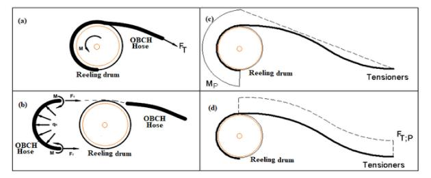
**Figure 6.** Hose-Pipe mechanics analysis in reeling operation on OBCH, (a) before spooling, (b) during spooling, (c) moment diagram during spooling-on in reality and (d) shear force diagram during spooling-on in reality.
