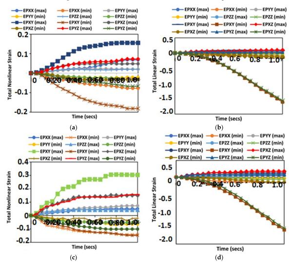
**Figure 9.** The total strain profiles for the reeling hose epoxy composite model. (a) total nonlinear strain of carbon fibre linear elastic model, (b) total linear strain of carbon fibre linear elastic model, (c) total nonlinear strain of epoxy elastoplastic model.
