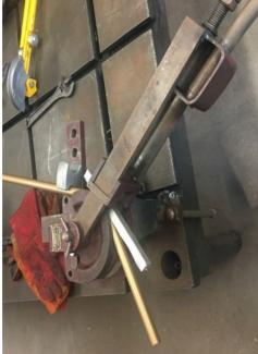
**Figure 1.** An application of tubular pipe bending using two methods conducted in Lancaster University Engineering Workshop.
