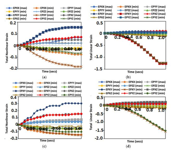
**Figure 10.** The total strain profiles for the reeling hose Carbon fibre composite model, showing (a) total nonlinear strain of carbon fibre linear elastic model, (b) total linear strain of carbon fibre linear elastic model, (c) total nonlinear strain of carbon fibre elastoplastic model, (d) total linear strain of carbon fibre elastoplastic model.
