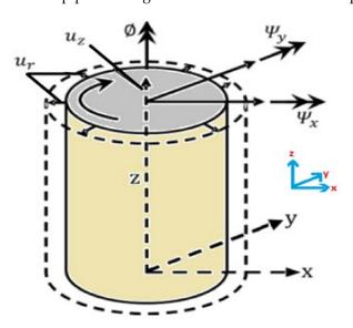
**Figure 4.** Sign conventions for the cylindrical layer of tubular pipe showing force and deformations.
