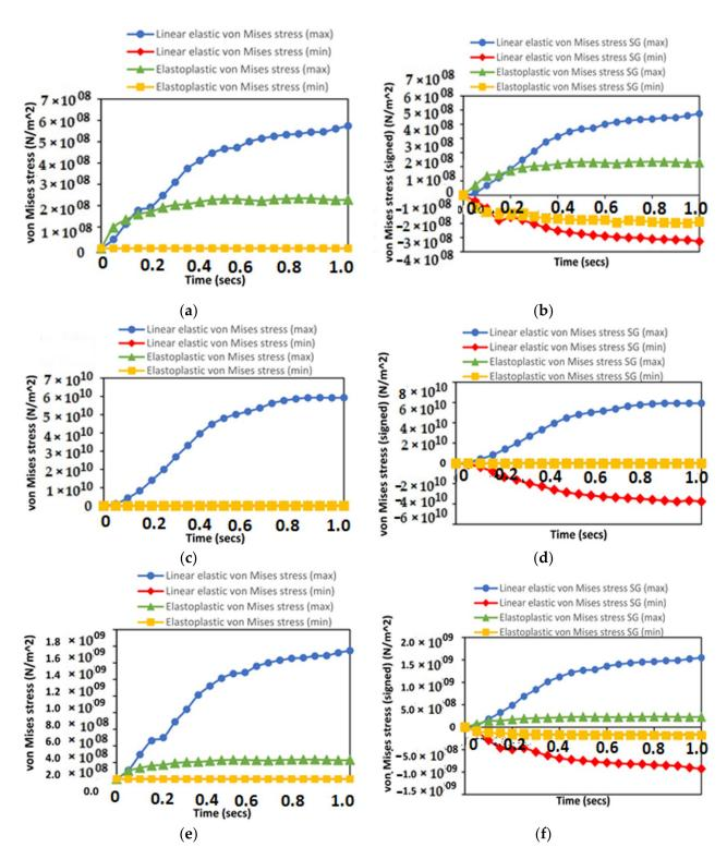
**Figure 12.** The stress profiles for the (a) von Mises stress on epoxy composite, (b) von Mises stress (signed) on epoxy composite, (c) von Mises stress on carbon fibre composite, (d) von Mises stress (signed) on carbon fibre composite, (e) von Mises stress on Nylon PA66-GF glass fibre composite models and (f) von Mises stress (signed) on Nylon PA66-GF glass fibre composite models.
