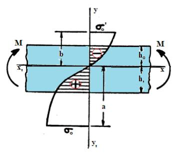
Figure 3. Plastic bending showing moments.
