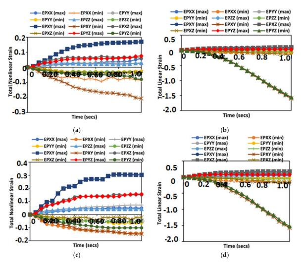
**Figure 11.** The total strain profiles for the reeling hose Nylon PA66GF composite model, showing (a) total nonlinear strain of nylon PA66GF linear elastic model, (b) total linear strain of nylon PA66GF linear elastic model, (c) total nonlinear strain of nylon PA66GF elastoplastic model, (d) total linear strain of nylon PA66GF elastoplastic model.
