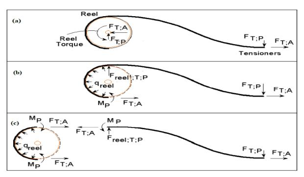
**Figure 7.** Forces on the **(a)** hoseline and the reel during spooling-on in reality, **(b)** hoseline during spooling-on in reality and **(c)** mechanical system for hose and reel separately for spooling-on.
