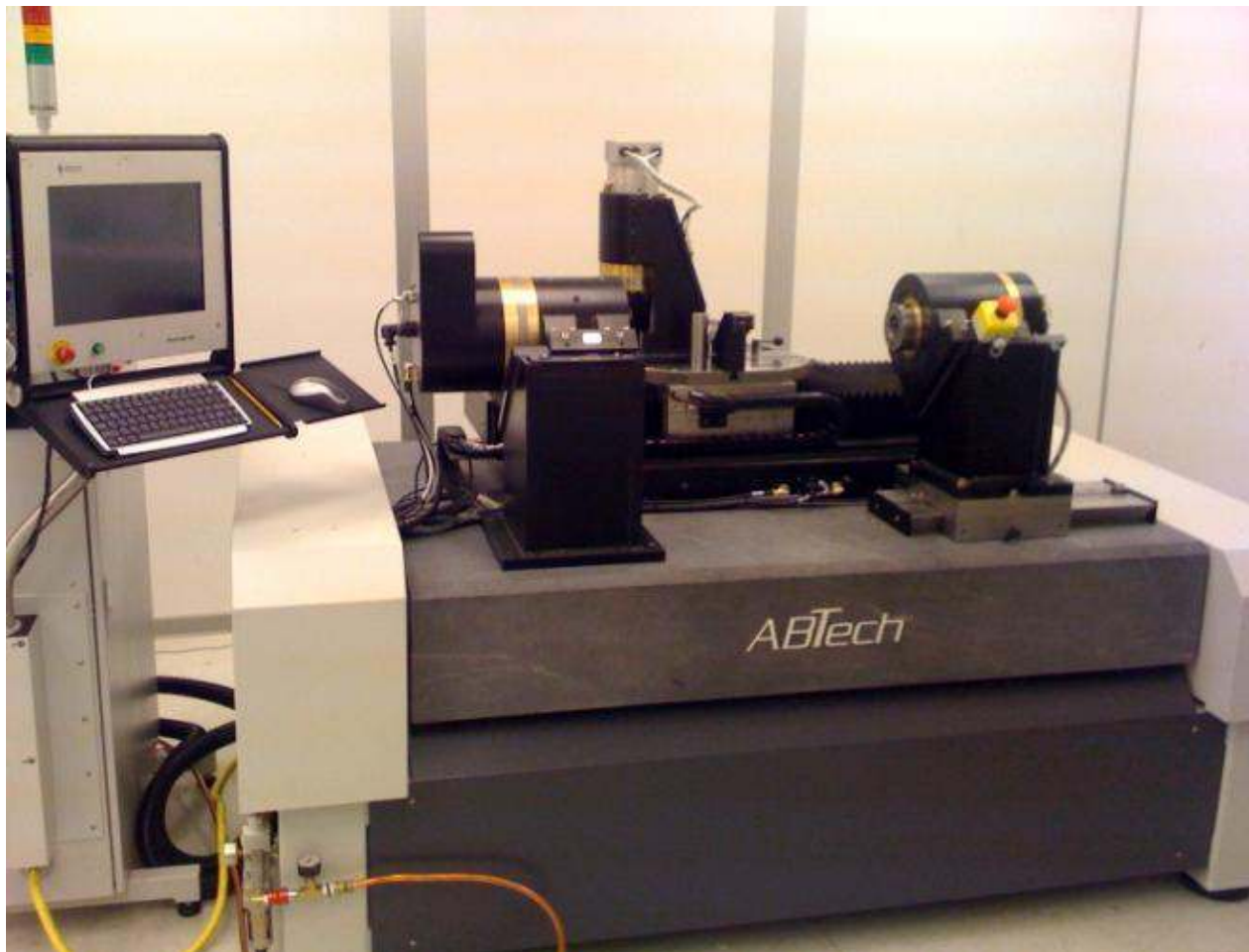
Figure 4: NuSTAR assembly machine installed inside a class 1000 clean room at Columbia University's Nevis Laboratory.
