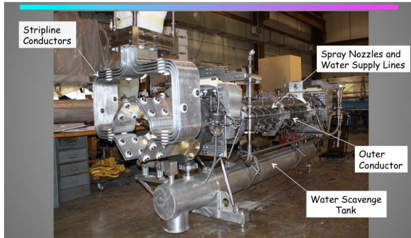
Figure 33. NuMI Horn 1 ready spare.
