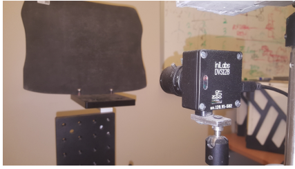
Fig. 5. DVS128 sensor used in our experiment for data collection. In each data collection experiment, the sensor was kept under constant illumination in an empty room isolated from any activity.
