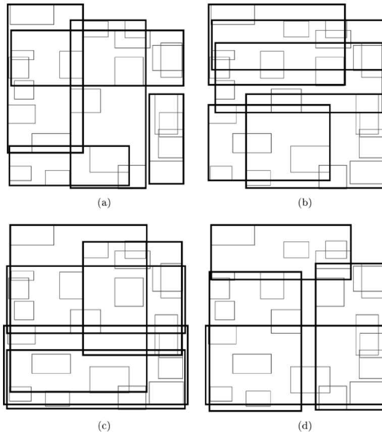
Fig. 20. The bounding boxes corresponding to the first level of aggregation for an R-tree built using different node splitting policies: (a) exhaustive, (b) linear, (c) quadratic, and (d) the linear algorithm of [Ang and Tan 1997] for the collection of 22 rectangles in Figure 14.
