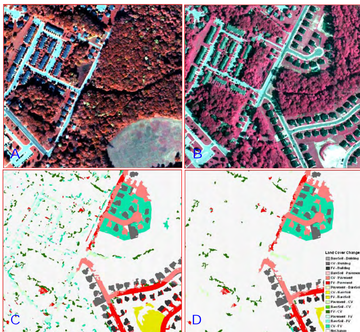
Figure 8. A comparison of the change detection results of the same landscape using the two different approaches: the pixel-based post-classification comparison (Panel C) and the object-based post-classification comparison (Panel D). Panel A shows the 1999 Emerge image for the landscape, while Panel B shows the one for 2004.
