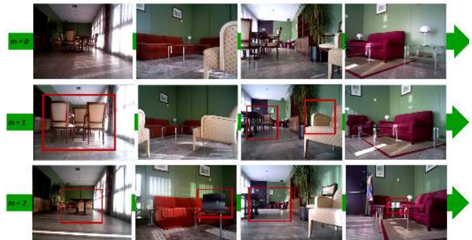
Fig. 4. Sample of images captured by the robot in three different mapping sessions. Changes as movement of chairs, presence of new objects such as cups or bottles are introduced between mapping sessions (red boxes).
