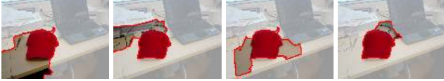
Figure 3. Some samples of the object candidates obtained with [14]. It can be seen that candidates within an image may have substantial overlap.
