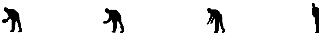
Fig. 11. VOPs used on a test ( VOP_{109}, VOP_{113}, VOP_{126}, VOP_{140} from left to right). VOP_{109}, VOP_{113} , and VOP_{126} represent bending instances, while VOP_{140} shows an almost standing body. Note that VOP_{126} , which has separate arms, results in a large distance from VOP_{109} in the case of the Fourier descriptor.
