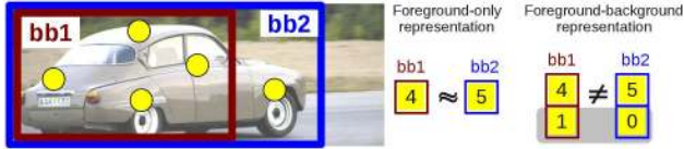
Fig. 4. Bounding boxes bb_1 and bb_2 have a similar foreground-only feature representation, but they are very different under the foreground-background representation. Here, the numbers denote the count of object-related descriptors. For bb_1 , parts of object that leaked into the background will be greatly discounted by the background model.
