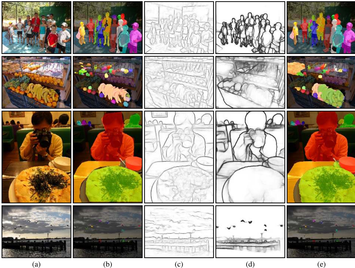
Figure 12. Example results on MS COCO val2014. In each row from left to right we present (a) input image, (b) ground truth annotation, (c) edge detection [13], (d) our object contour detection and (e) our best object proposals.
