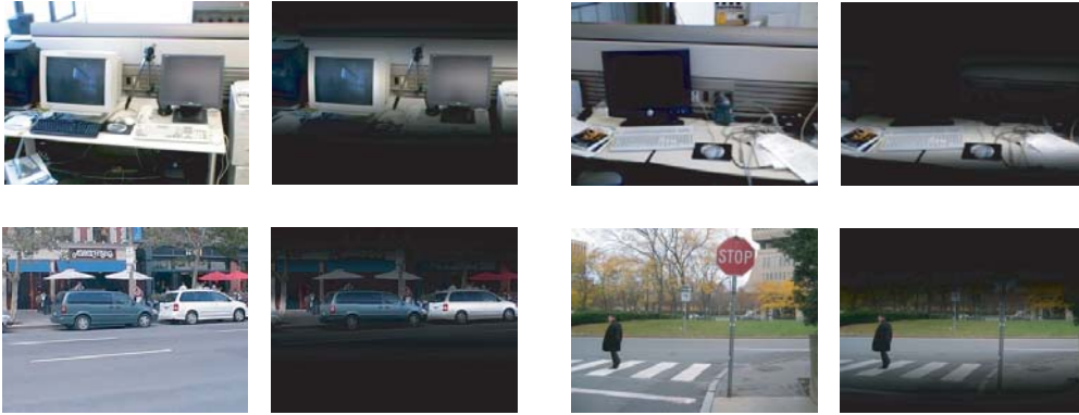
Fig. 8. Example of location priming for screens, keyboards, cars and people using global features. In each group, the image on the left is the input image, and the image on the right is the input image multiplied by the probability, given the gist, of the object being present at a given location, i.e., I. * P(x|G(I)) .
