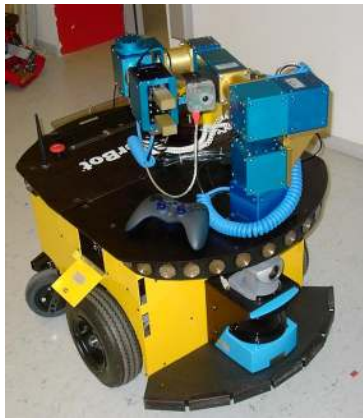
Figure 2: The experimental platform: PowerBot from MobileRobots Inc.
