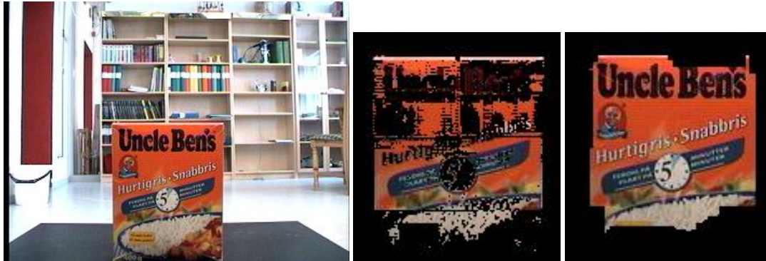
Figure 5: Left: The original image. Center: The result after simple image differencing (only a part of the image is shown). Right: The result after morphological operations.
