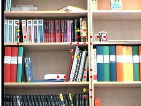
Figure 6: An example of the greedy search strategy used while searching for the cup at the intermediate zoom level. Squares represent possible object locations, and crosses are the calculated zoom locations that cover all the hypotheses. There are 4 zoom locations and 30 hypotheses in this example.
