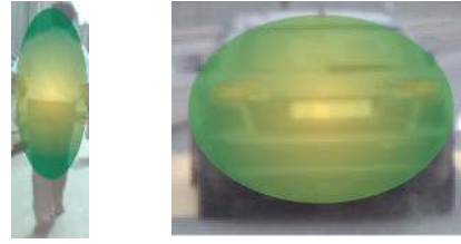
Fig. 3 Colour histograms are calculated inside an ellipse fitted to the bounding box, weighted with a Gaussian.
