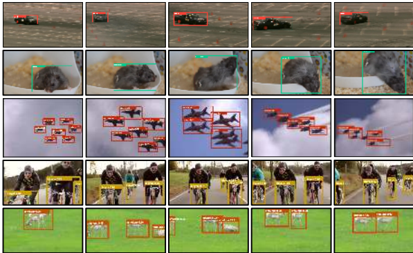
Figure 5. Qualitative results on the ImageNet VID dataset. The bounding boxes are tight and stably concentrate on the objects since the RoIs for each frame are based on the predicted locations on the previous frame. The last 3 rows show the robustness to handle scenes with multiple objects.)
