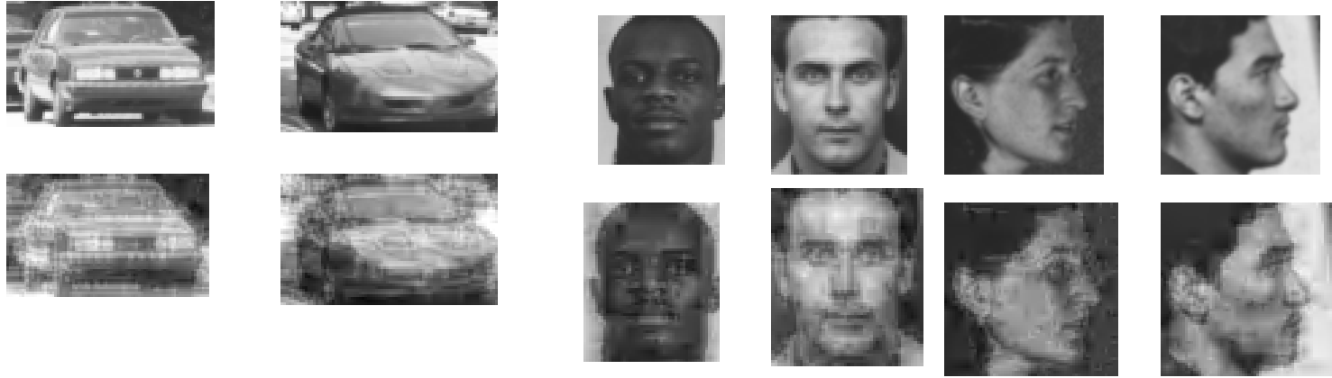
Figure 8: Images reconstructed by inverse wavelet transform. All wavelet coefficients in LH and HL bands were quantized to three levels per coefficient
