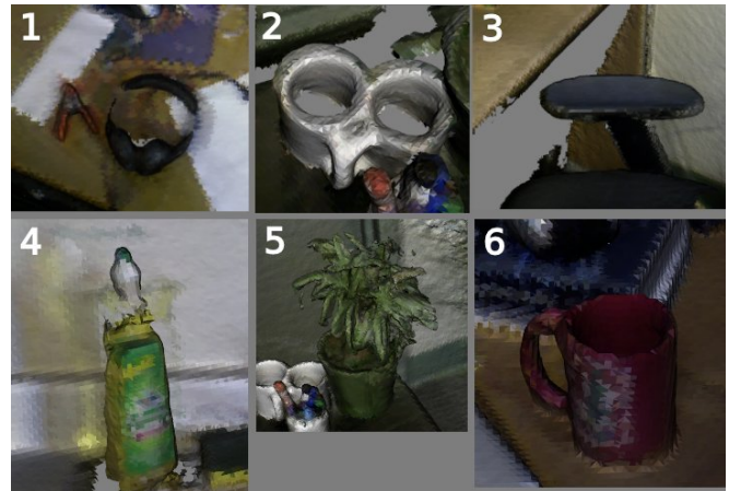
Fig. 8. Examples of limitations. 1: Only main part of the headphones will be identified as a candidate object. 2: Cups are fused and get segmented together as a single object candidate. 3: The armrest of the chair will be incorrectly identified as a strong object. 4: Due to transparency, the top will appear to be floating and gets disconnected from the bottle. 5: The plant is too intricate and contains too much variation to be selected as a single object. 6: The interior of the cup will be selected as a separate segment because the curvature changes too quickly around its rim.
