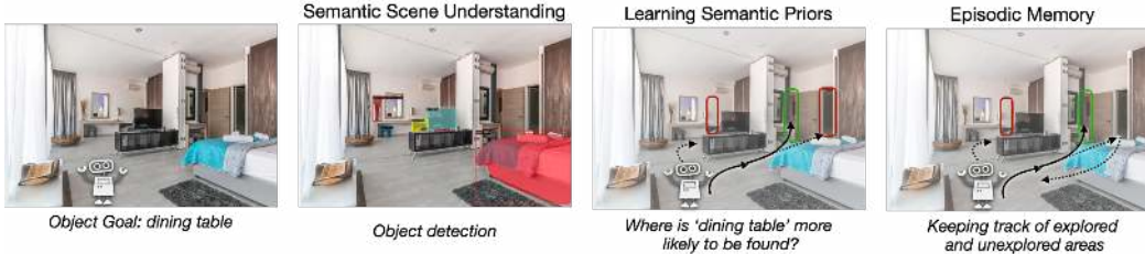
Figure 1: Semantic Skills required for Object Goal navigation. Efficient Object Goal navigation not only requires passive skills such as object detection, but also active skills such as building an episodic memory and using it effectively to learn semantic priors about relative arrangements of objects in a scene.
