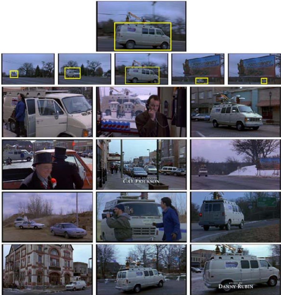
Fig. 10. Object level video matching I. Top row: The query frame with query region (side of the van) selected by the user. Second row: The automatically associated keyframes and outlined query regions. Next four rows: Example frames retrieved from the entire movie ‘Groundhog Day’ by the object level query. Note that views of the van from the back and front are retrieved. This is not possible with wide-baseline matching methods alone using only the side of the van visible in the query image.
