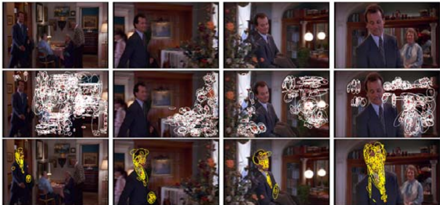
Fig. 8. Example IV: object level grouping for another (645 frame) shot from the movie Groundhog Day . Top row: The original frames of the shot where a person walks across the room while tracked by the camera. Middle and bottom row: The two dominant (measured by the number of tracks) objects detected in the shot. The number of tracks associated with each object is 401 (the walking person) and 15,053 (background). The object corresponding to the walking person is a join of three objects (of size 114, 146 and 141 tracks) connected by a long range repair using wide baseline matching, see figure 9b. The long range repair was necessary because the tracks are broken twice: once due to occlusion by a plant (visible in frames two and three in the first row) and the second time (not shown in the figure) due to the person turning his back on the camera. The trajectory of the regions is not shown here in order to make the clusters visible.
