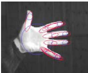
Figure 8. Feature extraction: Extracted blobs and ridges at appropriate scales.
