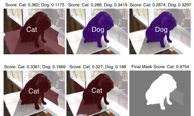
Fig. 7 (Best viewed in color) An image of a cat from the VOC2009 dataset. We show the cat/dog scores of the 5 top scoring segments from the image. It is relatively difficult to distinguish if this instance is a cat or a dog, from the foreground/object information only (e.g., top-middle and top-right segments). However, our algorithm takes advantage of multiple slightly different overlapping segments to produce a robust decision, that consistently improves upon the simple decision rule. In the Final Mask, the cat itself has the strongest score (indicated by high intensity values)
