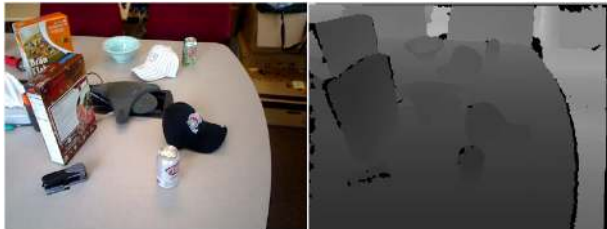
Figure 3. RGB and Depth image captured by an RGB-D camera. The black pixels in the right image are missing depth values.
