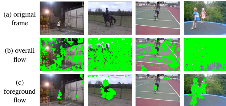
Fig. 2. The videos include an extensive amount of camera motion, thus, uneven flow fields. We use a homography based approach to estimate the flow of the foreground objects, following [21]. (a) shows the original frames from four videos. (b) shows the flow estimate (in green) without the motion stabilization. (c) shows the foreground flow estimate obtained following stabilization. As seen, this estimate gives us the ability to concentrate on the moving foreground objects.
