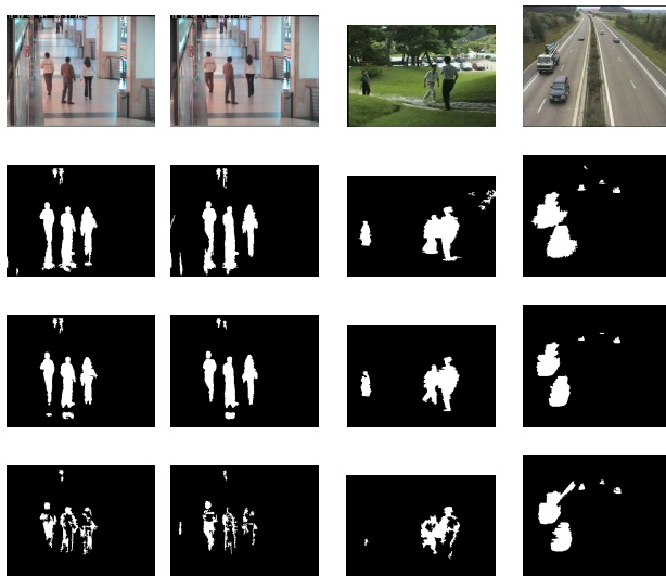
Figure 7. Segmentation results. The top row shows the original frame. The second row shows the results from the MoG implementation of [5]. The third row shows the results obtained with CMoG. Finally, the fourth row shows the results with CKDE.
