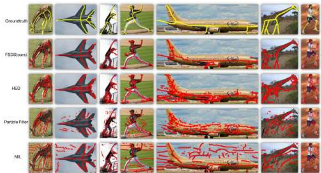
Figure 7. Illustration of skeleton extraction results on the SK506 dataset for several selected images. The groundtruth skeletons are in yellow and the thresholded extraction results are in red. Thresholds were optimized over the whole dataset.
