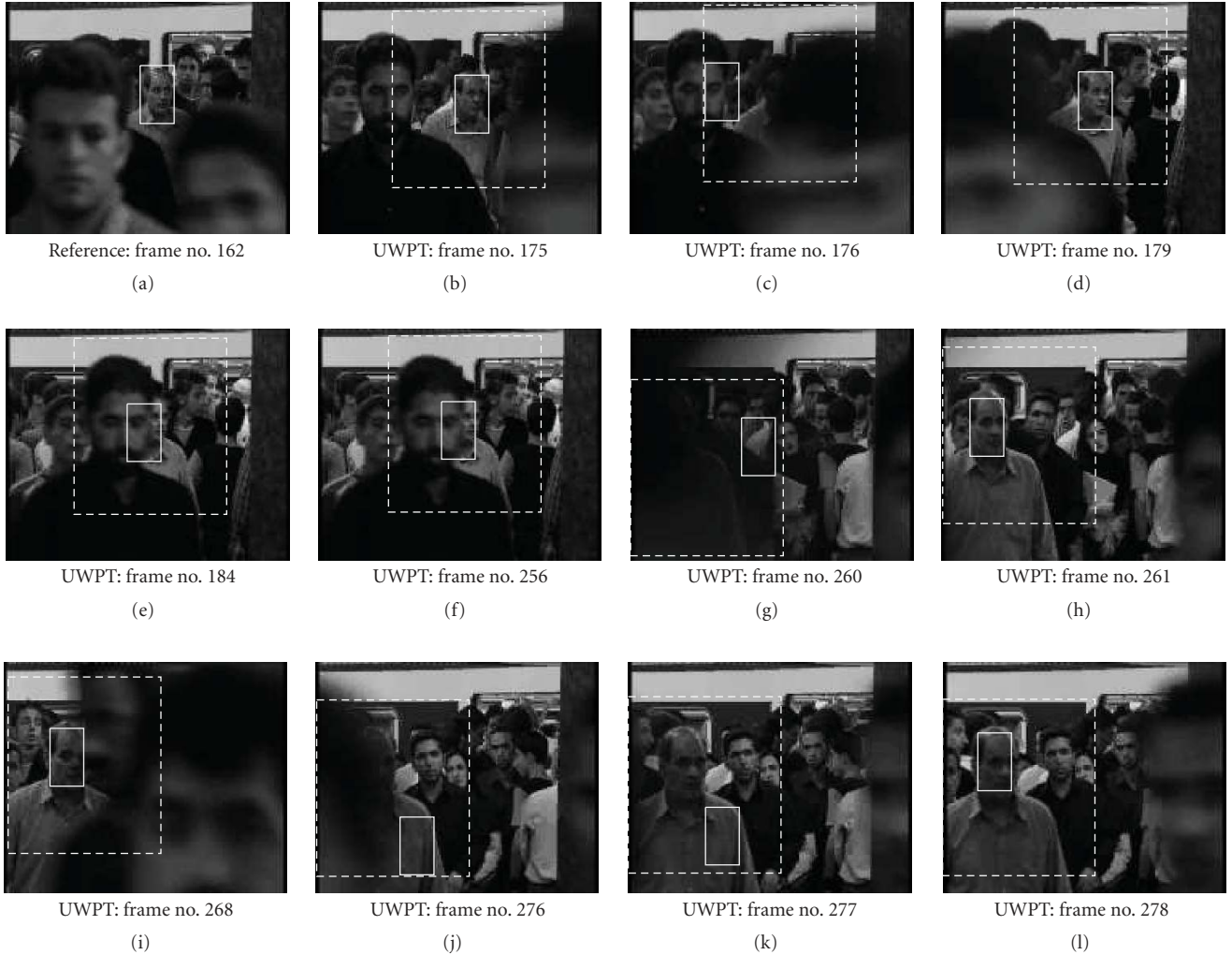
FIGURE 9: A man is tracked in the crowd in the metro in the presence of partial and full occlusions and zooming effects (all figures are the results of the proposed algorithm).
