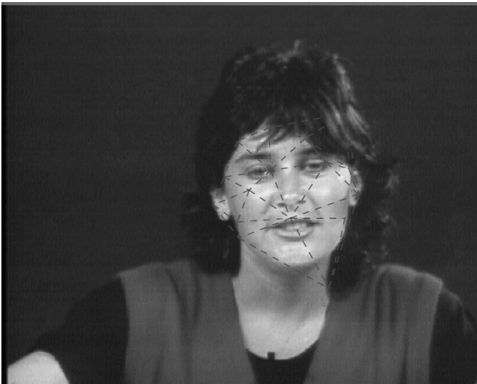
Fig. 8. Tracking result of the 100th frame of the Miss America sequence by independent node-point matching.
