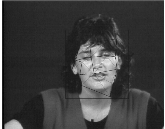
Fig. 6. Tracking result of the 100th frame of the Miss America sequence tracked by the proposed method (mesh) and the method of [11] (block).
