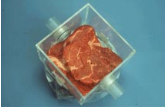
Figure 1. Setup of the sirloin steak in the rotation device.
