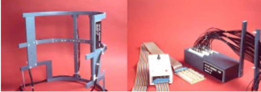
Figure 3. Brainwash fixation aid. Top: View of fixation aid with ends of optic fibers (all of them illuminated for clarity). Note the optic fibers exiting from the back of the device. Bottom: view of sequencer box (left) connected to a bank of LED's (center) that fits under the fiber optic bank (right).
