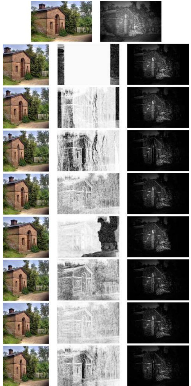
Fig. 6. First row: reference image and its saliency map. Second to last rows: retargeted images (left), SSIM maps (middle), and product of SSIM and saliency maps (right). Retargeted images from the second to last rows are generated by CR, MO, SC, SCL, SM, SNS, SV, and WARP algorithms, respectively.
