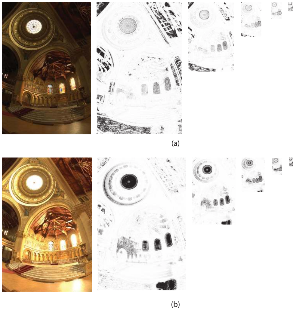
Fig. 2. Tone-mapped LDR images and their structural fidelity maps in five scales. The images were created using Adobe Photoshop “Highlight compression” and “Exposure and Gamma” methods (not optimized for quality), respectively. (a) S = 0.9152 ( S_1 = 0.8940 ; S_2 = 0.9341 ; S_3 = 0.9428 ; S_4 = 0.9143 ; S_5 = 0.8277 ). (b) S = 0.8614 ( S_1 = 0.9161 ; S_2 = 0.9181 ; S_3 = 0.8958 ; S_4 = 0.8405 ; S_5 = 0.7041 ).
