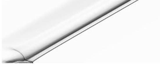
FIGURE 4. To illustrate the features of the process, we show an early phase of the oblique shock implosion shortly after the conical diaphragm has burst. The dispersed expansion wave that propagates to the upper left is visible as a broad grey band. The shock wave that propagates to the bottom right, toward the axis of symmetry is seen as a sharp black line followed by the black contact surface just above it. The faint white line marks the original location of the diaphragm.
