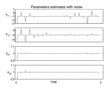
**Figure 3:** Parameters estimates for the nonlinear observer approach: estimation of four parameters in presence of noise.
