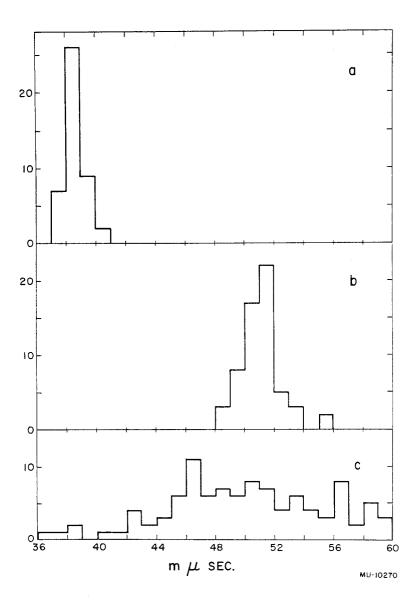
Fig. 3. (a) Histogram of meson flight times used for calibration.(b) Histogram of antiproton flight times.
