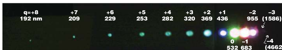
Fig. 3. Photograph of the Raman sidebands (projected onto a fluorescent sheet and taken by a CCD camera). The wavelengths calculated with Eq. (1) are also shown. The third and fourth Stokes sidebands shown in parentheses are observed only by the pyroelectric energy and/or MCT detector. The photograph contrast and light level from q = 2 to q = 8 are enhanced for a clear view. Apparent variation in the spot sizes is due to over-exposure while distortion from the straight line (around q = 6-8 ) is caused by bending of the fluorescent sheet.
