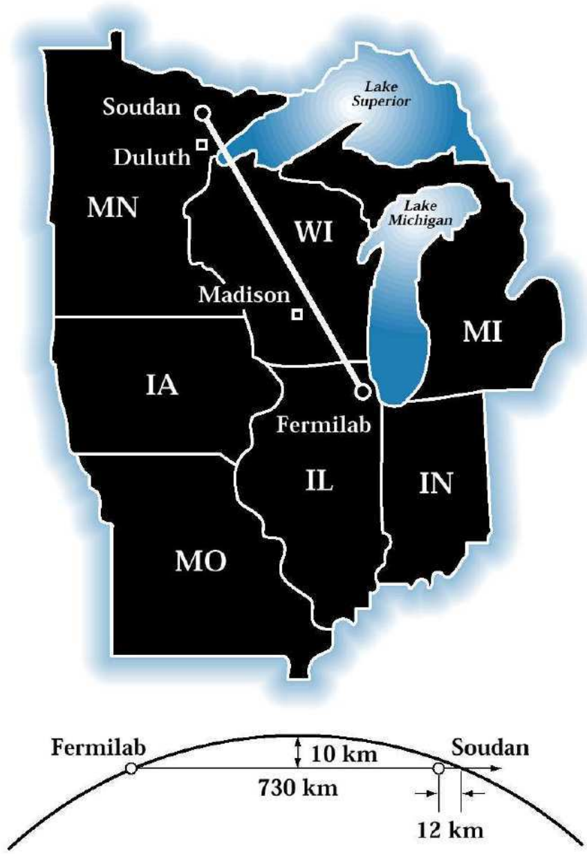
Figure 2.1: A geographical layout of MINOS detectors. The source of neutrinos for MINOS experiment is Fermilab's NuMI beam-line. The beam is steered toward the two MINOS detectors. The Near Detector (ND) is located close to the source of neutrinos on Fermilab site, while the Far Detector (FD) is 735 km away in the Soudan mine, Minnesota. Figure taken from [32].
