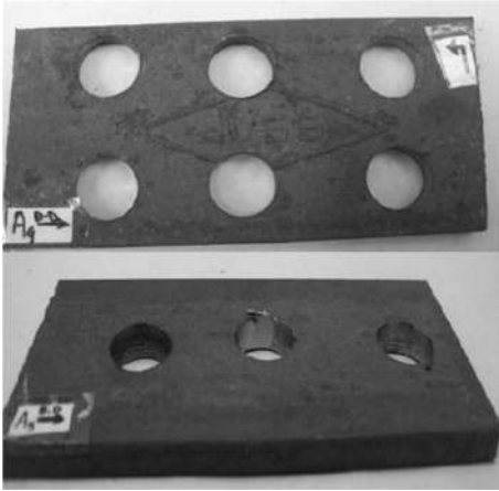
FIGURE 8: Photographic view of burr formed in experiment set III (left-right order: middle for Sl. numbers 1–3, top for Sl. numbers 4–6, bottom for Sl. numbers 7–9).
