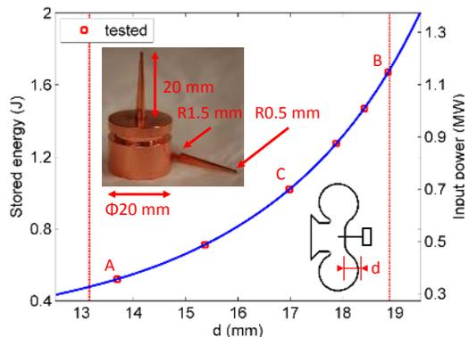
FIG. 1. Stored energy inside the cavity and input power for the same  $E_{tip}$  (625 MV/m) at different cathode positions. The red vertical lines show the cathode position boundaries in the experiment. Inset: pin cathodes from SLAC.
