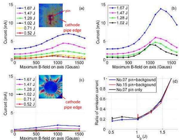
FIG. 5. (a-c): Captured dark current of the No.07 and No.15 pin cathodes at  $E_{tip}$  of 625 MV/m, and the flat cathode with different stored energies in the cavity. (d): Relative dark current with different stored energies. Insets of (a) and (c): dark current images with the pin and the flat cathode taken at the second cross (C2 as shown in Fig. 3).
