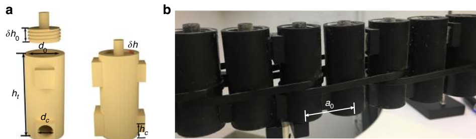
Fig. 1 1D tunable acoustic quasicrystal. a Schematics of a single resonator with a piston. b Photograph of 8 (out of 37) tunable resonators of the fabricated quasiperiodic acoustic crystal. The maximum height of a single cylinder in Fig. 1a is chosen as h_t = h_0 + \delta h_0 , where h_0 = 40 mm is the unperturbed height, \delta h_0 = 0.12h_0 is the modulation depth, and variable \delta h is modulated by the sinusoidal function in the range of [-\delta h_0, \delta h_0] . The diameter of cylinder d_0 = 20 mm. The connectors between the cylinders have a diameter d_c = 10 mm, with a vertical distance to the bottom of the hollow chamber h_c = 5.2 mm
