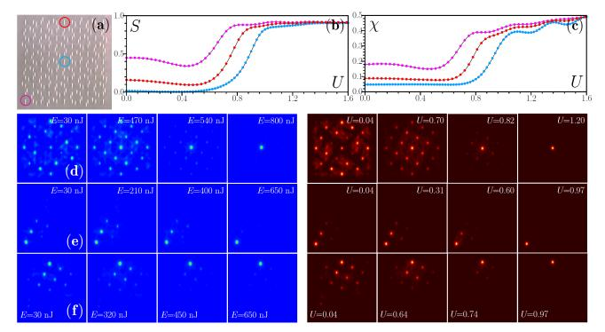
Fig. 3. (a) Photograph of the fs-laser written ML with  $\theta_1 = 0.2048\pi$ ,  $\theta_2 = 0\pi$ ,  $L = 11w_s$ . Theoretically calculated power fraction, which remains in the excited waveguides (b), and output form-factor (c) vs input power. Color coding for the lines correspond to circles in (a) indicating excited guides. Output experimental (blue images) and corresponding theoretical (dark-red images) distributions for the excitation in the center of ML
