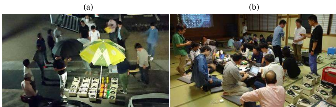
Photo 1 Snapshot during the 8th MRC. (a) Huddle tests. (b) Desktop study to identify peaks of the H/V spectrum ratios.
