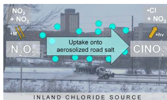
Figure 1. The role of road salt aerosol in wintertime \text{ClNO}_2 production in inland areas. Vehicular traffic causes lofting of road salt, providing a chloride-containing particle surface for \text{N}_2\text{O}_5 uptake, producing \text{ClNO}_2 at night. Upon sunrise, \text{ClNO}_2 photolysis leads to chlorine radical formation and \text{NO}_x recycling, linking the common deicing practice to wintertime inland air quality.
