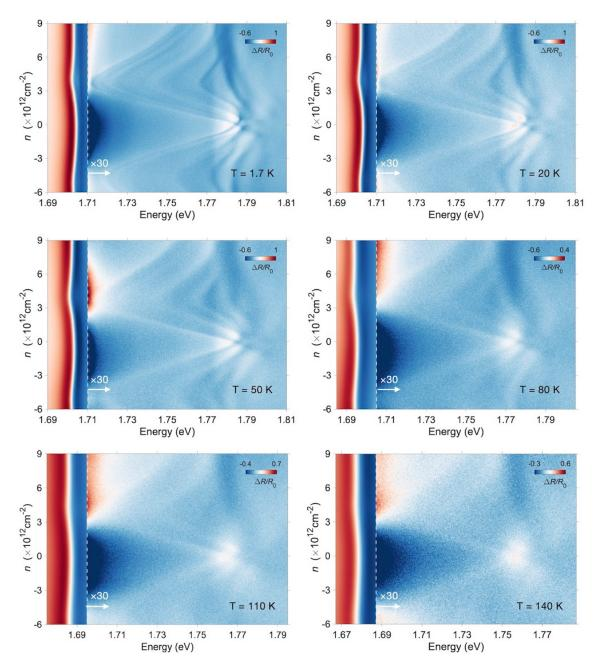
Fig. S2. Temperature dependence of the Rydberg moiré exciton. The lowest-energy branch of the  $X_{RM}$  survives to a temperature as high as ~140 K, in accordance with the large interlayer binding energies. The spectra for energies above the dashed lines are multiplied by a factor of 30 for clarity.
