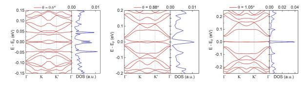
**Fig. S3. Calculated band structure (in red) and density of states (blue) of 0.6°, 0.88°, and 1.05° TBG.** The gap opening at the full filling vanishes at small twist angles (such as 0.6°).
