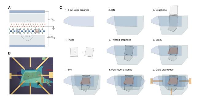
**Fig. S1. Device Fabrication.** (A to C), Device schematic (A), optical image (B) and fabrication process (C) of a typical device.
