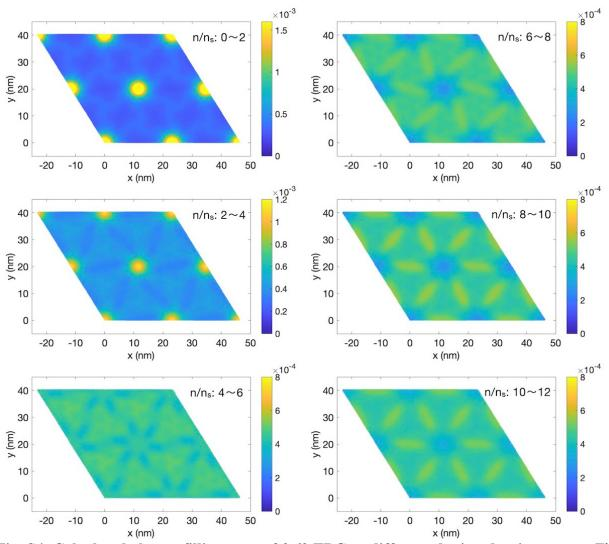
**Fig. S4. Calculated charge-filling map of 0.6° TBG at different doping density ranges.** The maps show the differences between the charge distribution at two values of  $n/n_s$ , which gives the charge-filling distribution in this range. At low doping densities (e.g.  $n/n_s < \sim 4$ ), the charges prefer to fill onto the AA sites (the regions in bright yellow). As the density becomes higher, the charges fill more onto the AB/BA stacked regions, with the less filled AA sites in dark blue.
