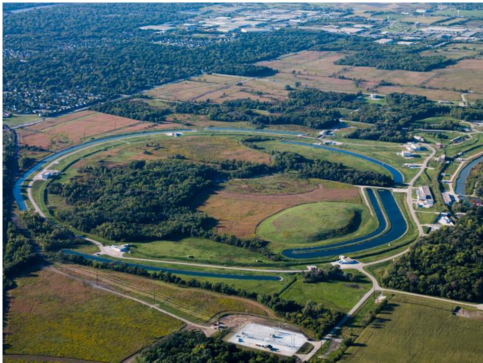
Figure 7: The Main Injector and the Recycler share the same tunnel, the later stores protons and antiprotons at the same time that provides additional cooling.
