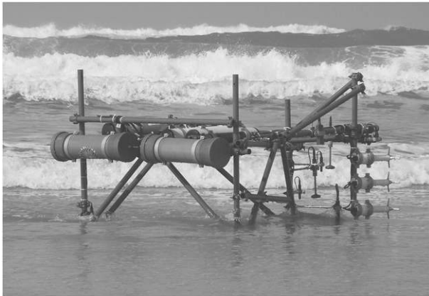
FIG. 1. Instrumented rig deployed at the neap low-tide water level during the ECORS Truc Vert 2008 experiment. The instruments were mounted on the northwestern side of the rig to ensure that the logging and power canisters did not influence the flow field at and the seabed below the sensors during conditions with waves from the west to northwest and with currents flowing southward (i.e., to the left in the image). The sensing volume of the upper of the three sideways-oriented ADVOs (the rightmost instruments in the image) is approximately 0.75 m above the seabed. The image was taken at low tide on 8 Mar 2008 (yearday 68).
