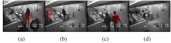
Figure 3. Examples of false alarms and abnormalities missed by our algorithm. (a)-(c) are false alarms; (d) is missed. (a) A person goes to the gate, and a person nearer to the camera is walking left to right. While this situation happens occasionally, here the nearer person slows down to talk, and the system raises an alert. (b) A person is getting on the train. Optical flows are often unreliable in the far-field areas, and it leads to a false alarm. (c) A person walks too fast. (d) Our method misses the “no payment action”, perhaps because the motion is very similar to passing through the gate normally. Best viewed in the electronic version.
