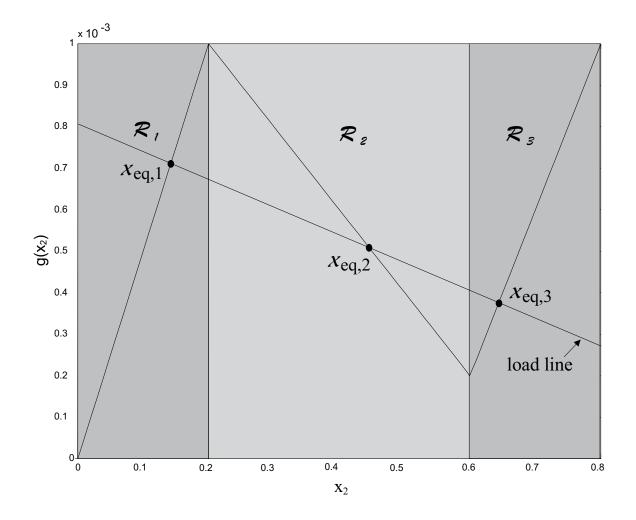
Figure 16: Tunnel Diode Characteristic for Example 4.
