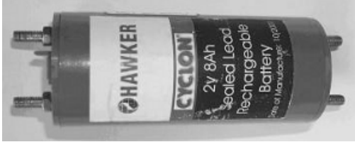
Fig. 3. 8Ah sealed VRLA test cell.
