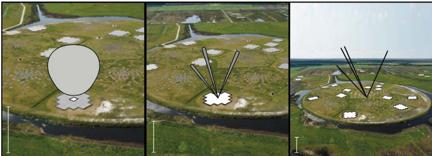
Fig. 1. Three successive zoom-outs showing the stations in the LOFAR core. The different scales of the hierarchically organised HBA elements are highlighted and their respective beam sizes are shown. The large circular area marks the edge of the Superterp, which contains the inner-most 6 stations (i.e. 12 HBA sub-stations: where there are 2 sub-stations, each of 24 tiles, in each HBA core station); other core stations can be seen highlighted beyond the Superterp in the third panel. Left: a single HBA tile and associated beam. Middle: a single HBA sub-station with three simultaneous station beams. Right: the 6 stations of the Superterp plus 3 core stations in the background are highlighted. Four independent beams formed from the coherent combination of all 24 core HBA stations, most of which are outside this photo, are shown. For the LBA stations, a similar scheme applies except that each LBA dipole can effectively see the whole sky. Fields of the relatively sparsely distributed LBA antennas are visible in between the highlighted HBA stations in all three panels.
