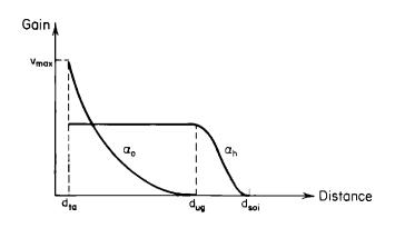
choosing the proper threshold, an additional method can be applied to minimize rank change effects. This is to consider obstacle avoidance only when sufficiently close to an obstacle, which would be compatible with limited-range proximity sensors. In order not to introduce a discontinuity, the obstacle avoidance term should be tapered as a function of distance.
