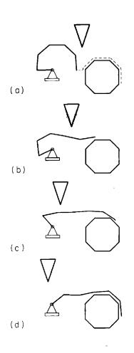
the manipulator. Inside of the  $d_{ug}$ , the influence of the obstacle in repelling the manipulator is inversely related to the distance. If the manipulator reaches the  $d_{ta}$ , then a collision is considered imminent and the specified task is suspended. This distance is determined by such factors as the maximum velocity and physical dimension of the manipulator, thus allowing the manipulator to slow down and stop before physical contact occurs.
